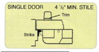
Grade 2 Fire Rim Exit Device - FIRE RIM EXIT DEVICE is a non-handed exit device with a dead
